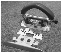
1. Three basic parts of your Trimmer: (Top to Bottom) Handle unit, locating plate and blade holder unit.
